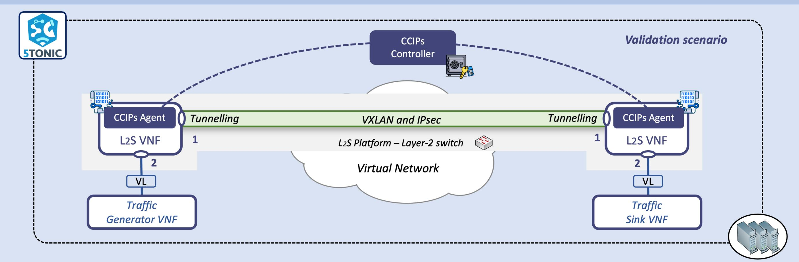
L2S platform offers an abstraction of a **layer-2 switch** with VLANs support that spans **multiple NFV sites**. In addition, it protects data communications among NFV sites using standards protocols and state-of-the-art open-source technologies (such as VXLAN, or IPsec), preserving isolated operations of multi-site NFV services.
